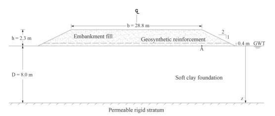
Figure 1 - Adopted embankment cross-section and foundation soil stratigraphy for the case study.
