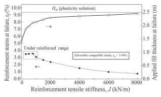
**Figure 9** - Effect of varying *J* from 300 to 8000 kN/m on the mobilized reinforcement strains at failure (closed circles, see left-hand side scale) and applied fill thicknesses at failure (open circles, see right-hand side scale) obtained by finite elements simulation of the case study.
