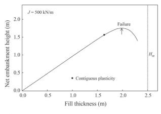
Figure 5 - Maximum net embankment height obtained by finite elements simulation of the case study with J = 500 kN/m.
