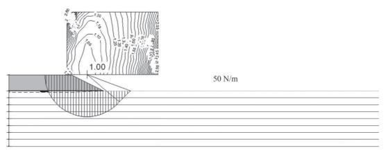
Figure 11 - Limit equilibrium stability analysis for factor of safety 1.0, allowing to estimate the required reinforcement force,  $T_{ro}$  (GGU Stability).
