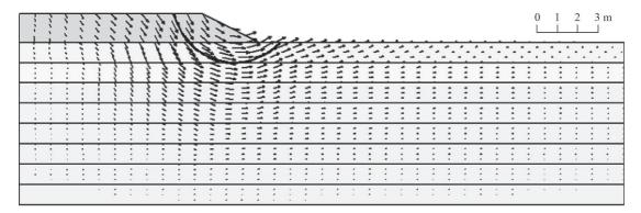
Figure 4 - Assessment of the embankment collapse height without reinforcement,  $H_c = 1.40$  m, using limit equilibrium, superimposed to finite elements vectors.
