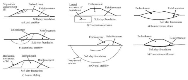
Figure 3 - Ultimate limit states for embankments on soft soils (modified from BS-8006, 2005).
