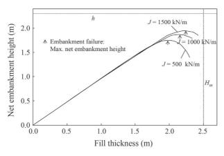
**Figure 7** - Effect of varying *J* from 500 kN/m to 1000 and 1500 kN/m on the maximum net embankment height obtained by finite elements simulation of the case study.
