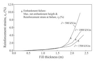
Figure 8 - Effect of varying J from 500 kN/m to 1000 and 1500 kN/m on the mobilized reinforcement strains obtained by finite elements simulation of the case study.
