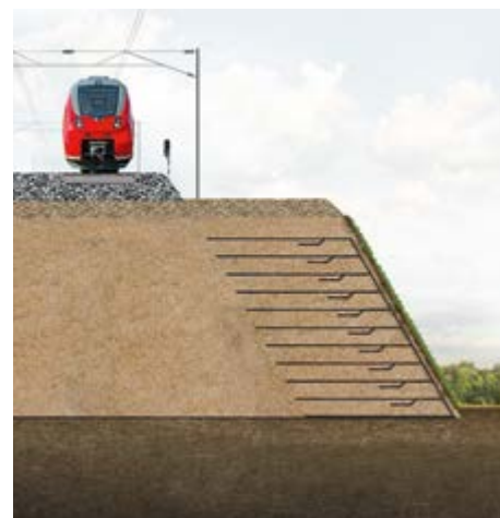
Retaining walls/steep slopes
