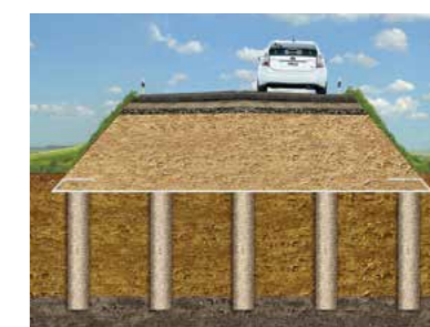
Pali in Geotessile Tubolare (GEC)
