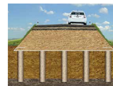
Pali in Geotessile Tubolare (GEC)
